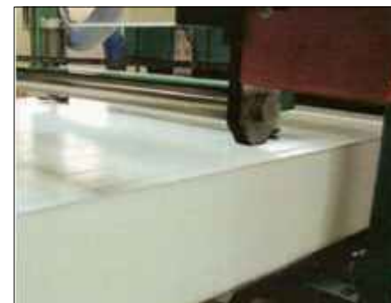
PFF insulated panels are produced on a fully automated, continuous line panel machine to achieve a superior thermal and structural building product
